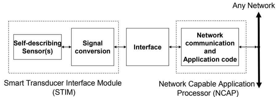
**Figure 1. IEEE-1451 Integrated Network Sensor Model**
