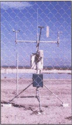
Meteorological data has been obtained from the CIMIS (California Irrigation Management Information System) database maintained by the California Department of Water Resources. CIMIS stations measure direct solar radiation, air temperature, relative humidity, and wind speed and direction. All measurements are reported hourly as averages for the preceding hour. There are four CIMIS stations located near the shores of the Sea (see basin map).
