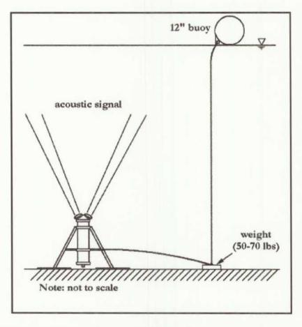
Each ADCP is completely self-contained with 30Mb of data storage and battery power sufficient for more than 80 days of recording data at 15 minute intervals.
