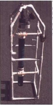
The Ocean Sensors Model OS200 CTD is self-contained and measures conductivity, temperature, and pressure. The instrument is deployed by dropping it through the water column from the boat. As it falls through the water column the instrument gathers data. It is then retrieved, and the recorded data is downloaded. The results are detailed profiles of water quality through the water column.
