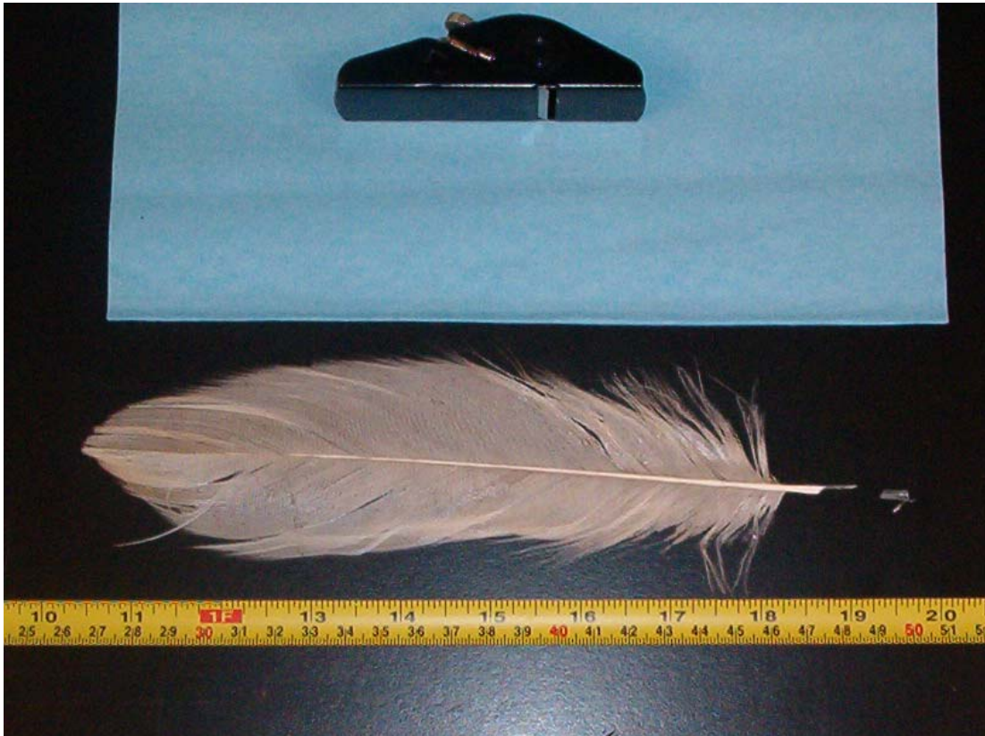
Figure 4. California Condor under-wing covert and cabinetmaker's plane used in preparation of feather samples for lead analysis.
