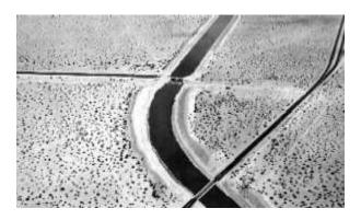
The Coachella Canal is a major branch of this system. Its turnout from the main canal is about 40 miles from Imperial Dam. The water flows by gravity about 70 miles north along the east margin of the Salton Sea to Indio, generally following the sea level contour. The canal curves west around Indio and terminates at the Lake Cahuilla reservoir at the base of the Santa Rosa Mountains. Completed in 1954, the 500-mile distribution network within the Lower
