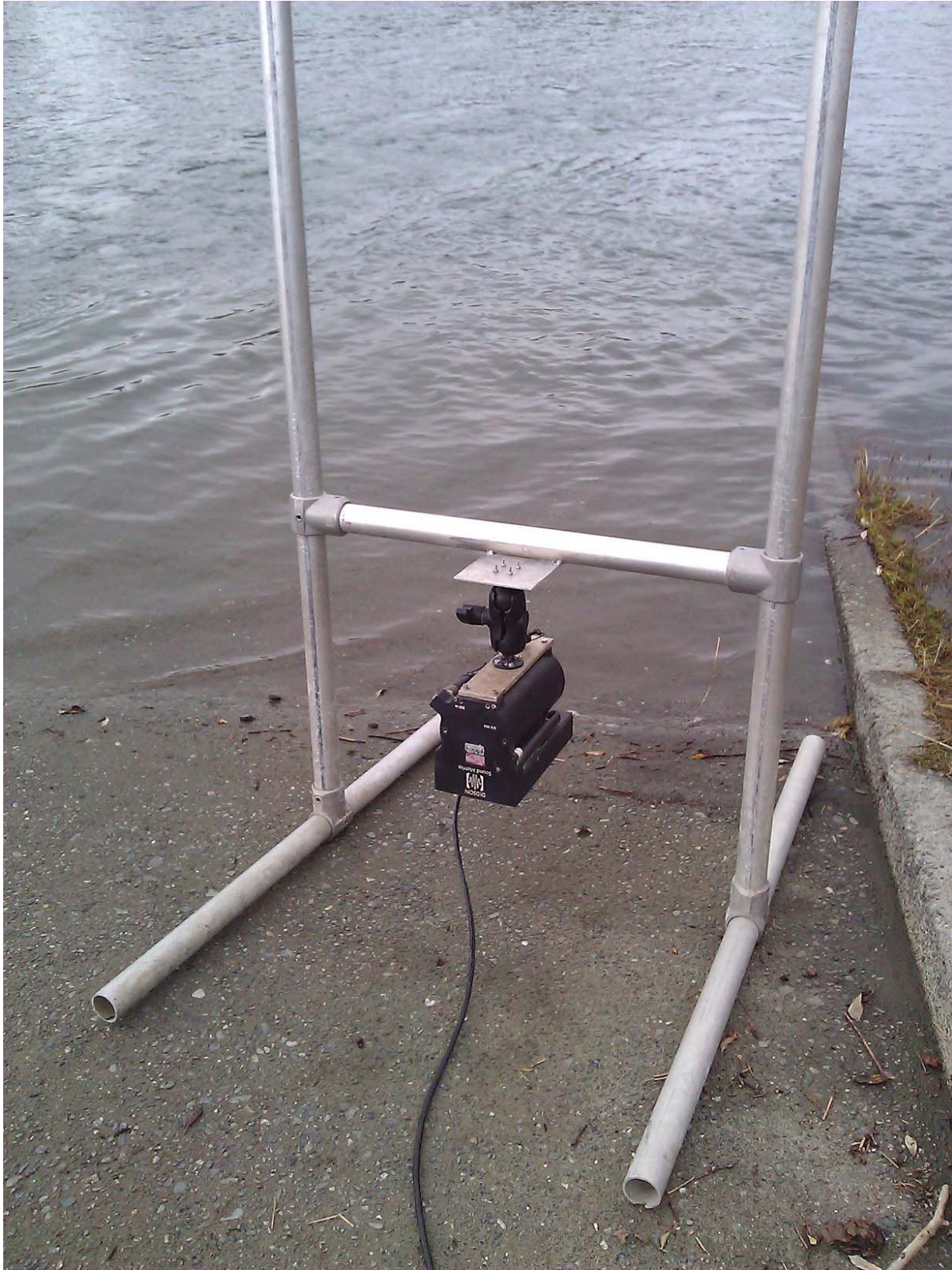
Figure 7. DIDSON H-Mount design constructed from aluminum pipe and fittings. The aluminum plate was fabricated and welded to the crossbar and attached to a RAM double socket ball joint to accept the DIDSON unit.
