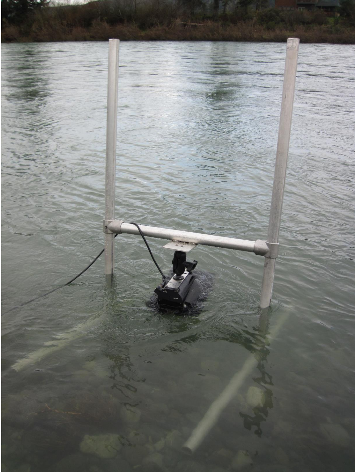
Figure 14. Left bank DIDSON deployment showing the large lens installed.
