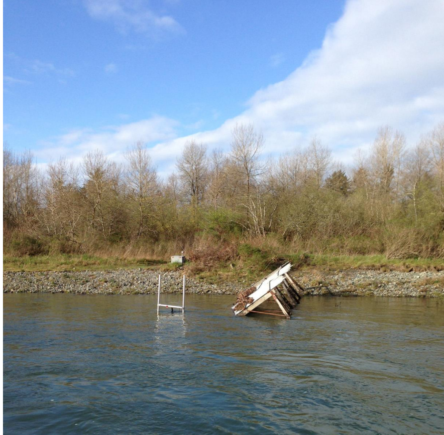
Figure 6. Left bank DIDSON showing the Alaskan Weir, H-Mount and remotely powered wireless communication box.
