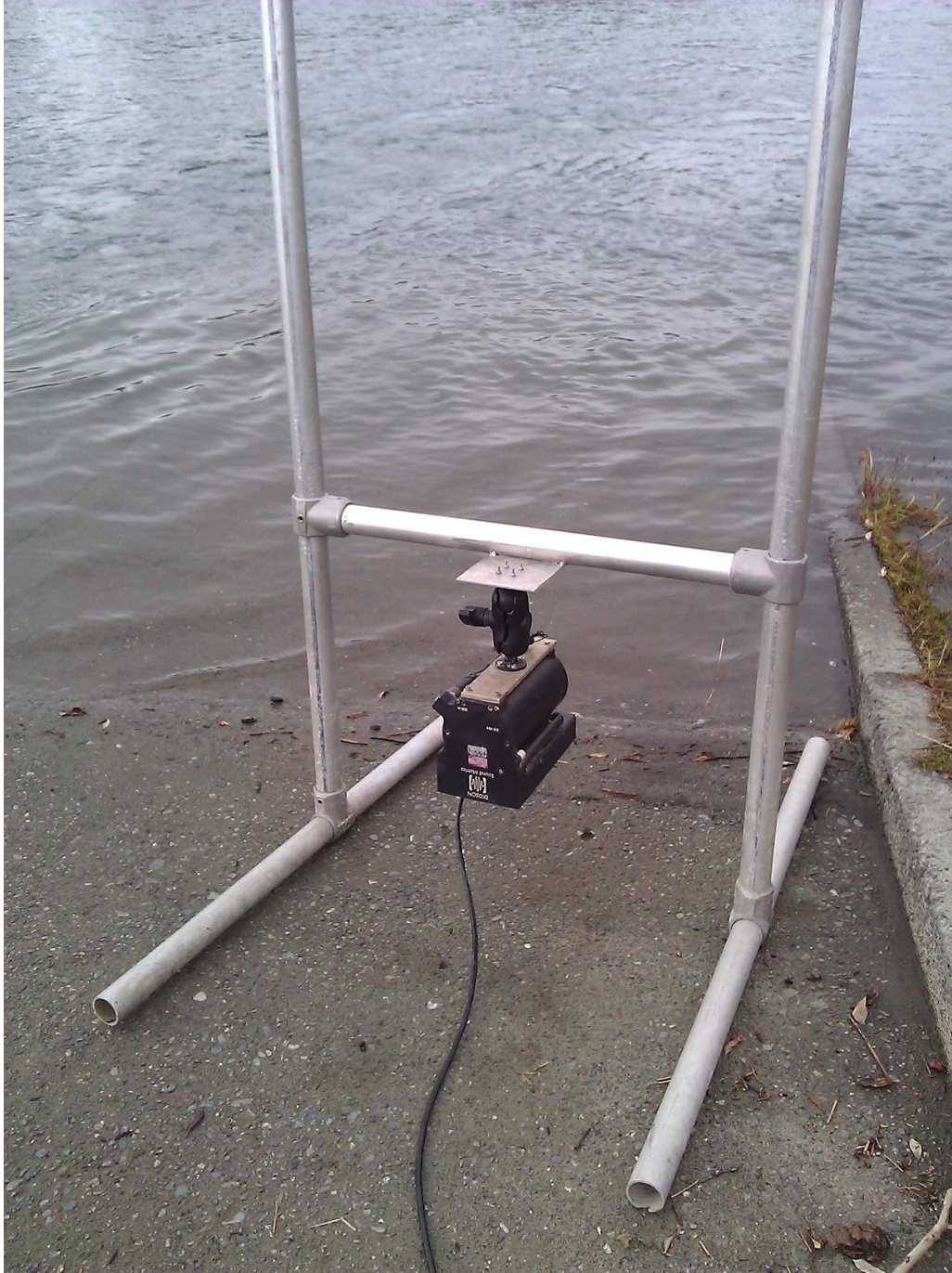
Figure 5. DIDSON H-Mount design for the Smith River right bank location constructed from aluminum pipe and fittings. The aluminum plate was fabricated and welded to the crossbar and attached to a RAM double socket ball joint to accept the DIDSON unit.
