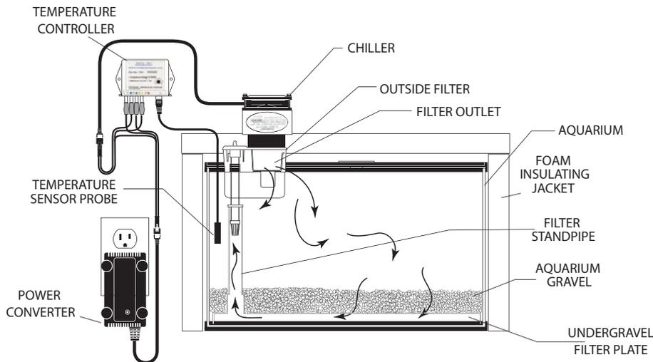
**Outside Filter System with temperature controller**
