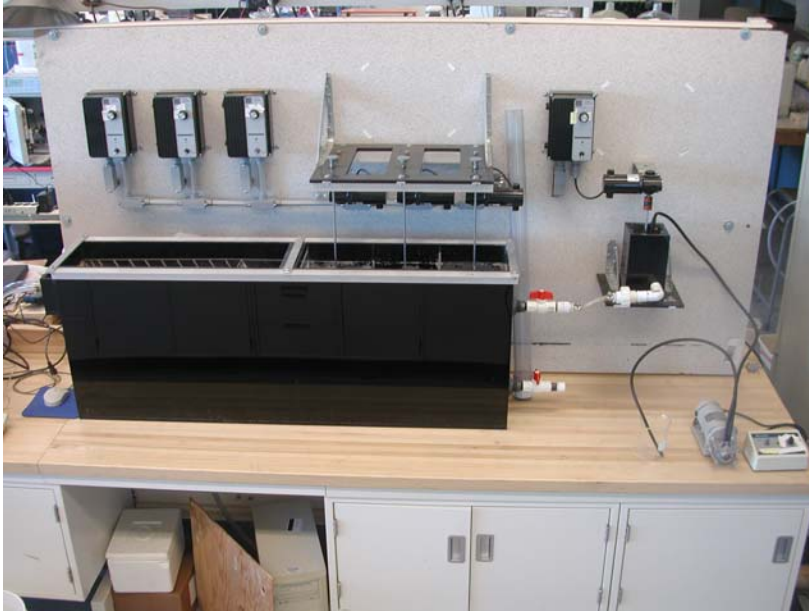
Photo 1. Dr. Matsumoto's coagulation, flocculation, sedimentation (CFS) unit
