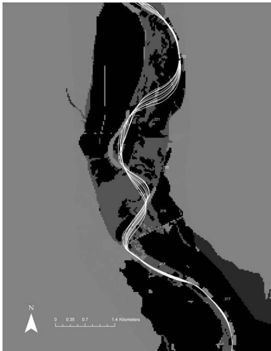
Woodson Bridge Shasta flow with existing revetment
