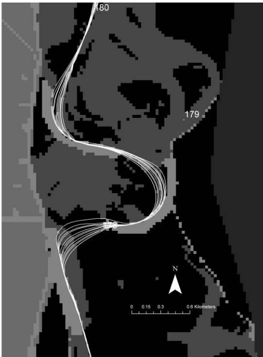
Ord Ferry Shasta flow with existing revetment
