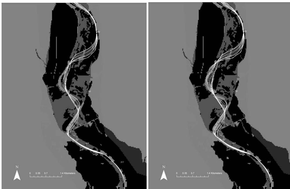
Figure 2-5. Predicted evolution of Woodson Bridge site for hypothetical flow scenario with existing (left) and altered (right) revetment conditions. Altered condition corresponds with revetment removal at RM 220–222 (right bank) at Kopta Slough.
