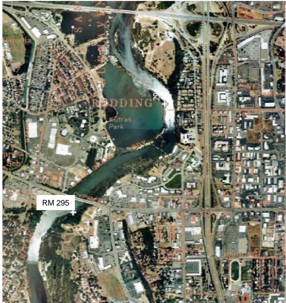
**Figure 2-2.** Lasting effects of aggregate extraction. Kutas Park (center) was one of the primary sources of aggregate for construction of Shasta and Keswick dams. Overall, more than 7 million cubic yards of sediment has been mined from the upper Sacramento River basin. Much of the mining has been done on the mainstem channel and floodplain. Remnant mining pits can trap sediment and disrupt the continuity of bedload transport. (Source: CDWR, 1999. Sacramento River Aerial Atlas.)
