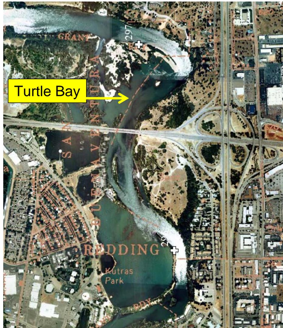
Figure 2-2. Lasting effects of aggregate extraction. Turtle Bay was one of the primary sources of aggregate for construction of Shasta and Keswick dams. Overall, more than 7 million cubic yards of sediment has been mined from the upper Sacramento River basin. Much of the mining has been done on the mainstem channel and floodplain. Remnant mining pits can trap sediment and disrupt the continuity of bedload transport. (Source: CDWR, 1999. Sacramento River Aerial Atlas.)
