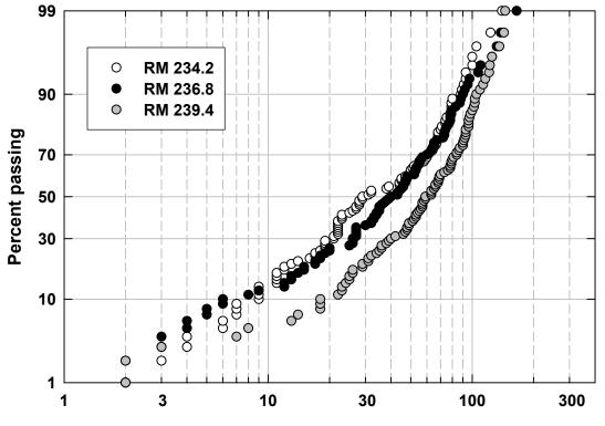
**Surface grain size (mm)---(from Wolman Counts)** Appendix Figure WC9. Grain-size distributions of the surface inferred from Wolman Counts at 3 locations on the Sacramento River in 2005. The Y axis shows a probability scale.
