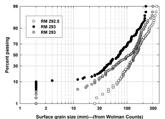
Appendix Figure WC3. Grain-size distributions of the surface inferred from Wolman Counts at 3 locations on the Sacramento River in 2005. The Y axis shows a probability scale.
