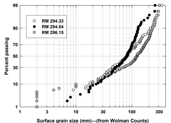
Appendix Figure WC2. Grain-size distributions of the surface inferred from Wolman Counts at 3 locations on the Sacramento River in 2005. The Y axis shows a probability scale.
