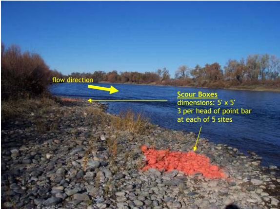
Figure 11. Scour boxes of the Sacramento River gravel study. Scour boxes dimensions were 5' x 5'. Three were installed at each of five sites in the study area. Scour box spacing was 20 m.
