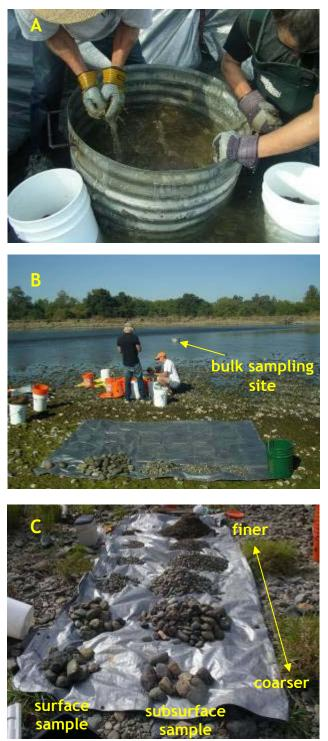
Figure 8. Bulk sampling of surface and subsurface bed samples from the Sacramento River. (A) A section of culvert (30 inch diameter) is worked into the bed and particles from the surface are extracted by hand. (B) Samples are sieved and the mass of each size class is recorded on a nearby bank. (C) Surface (left) and subsurface (right) samples, segregated into size classes for one of the samples from the middle Sacramento River.
