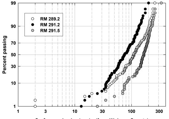
Surface grain size (mm)---(from Wolman Counts) Appendix Figure WC4. Grain-size distributions of the surface inferred from Wolman Counts at 3
