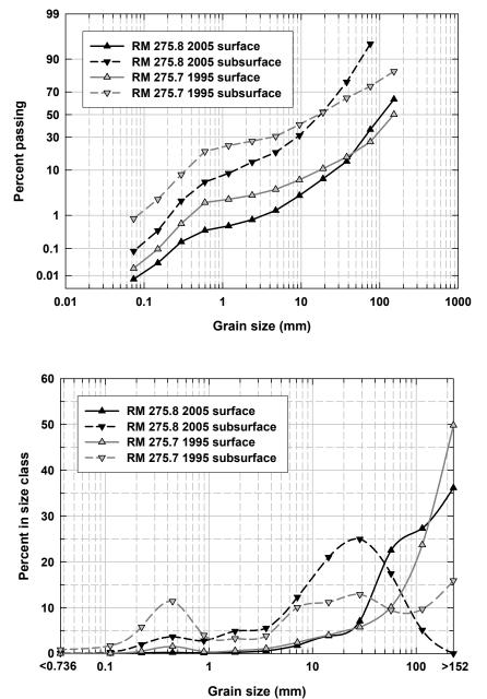
Figure 23. Time series of grain-size cumulative distribution functions (A) and probability distribution functions (B) of the surface (up-pointing triangles, solid line) and subsurface (down-pointing triangles, dashed line) at geomorphically comparable positions on a point bar at RM 275.7, based on data from bulk samples.
