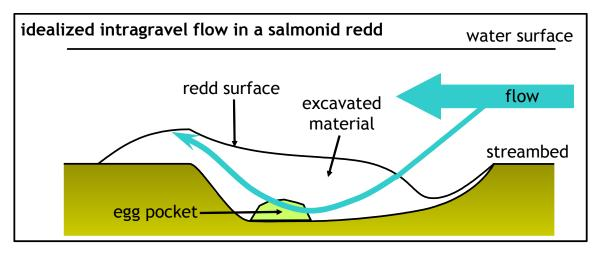
Figure 3. Conceptual diagram of intragravel flow through a buried salmonid egg pocket. The redd imposes a perturbation to the streambed profile, creating hydraulic conditions that force flow through the egg pocket.
