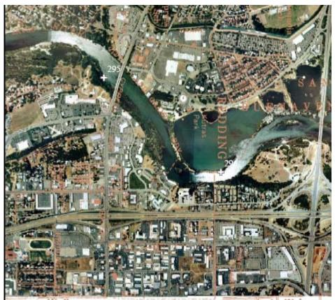
**Figure 1.** Lasting effects of aggregate extraction. Kutras Park (center) was one of the primary borrow areas for aggregate to support Shasta and Keswick dam construction. More than 7 million cubic yards of sediment was mined from the upper Sacramento River basin, much of it from the mainstem channel and floodplain. Remnant mining pits can function as sediment traps
