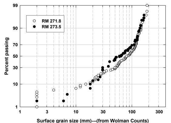
Appendix Figure WC8. Grain-size distributions of the surface inferred from Wolman Counts at 3 locations on the Sacramento River in 2005. The Y axis shows a probability scale.
