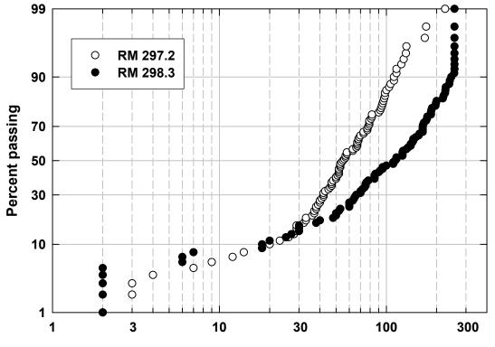
Surface grain size (mm)---(from Wolman Counts) Appendix Figure WC1. Grain-size distributions of the surface inferred from Wolman Counts at 2
