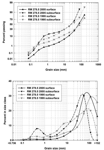
Figure 24. Time series of grain-size cumulative distribution functions (A) and probability distribution functions (B) of the surface (up-pointing triangles, solid line) and subsurface (down-pointing triangles, dashed line) at geomorphically comparable positions on a point bar at RM 278.5, based on data from bulk samples.
