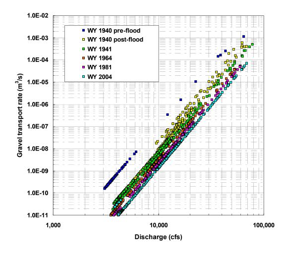
Figure 55. Sediment rating curves from TUGS model simulations at RM 294. The shift in the curves over time is a direct result of coarsening, which reduces bed mobility and thus reduces the predicted amount of sediment transport that should occur for a given flow.
