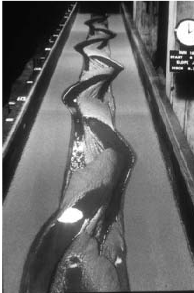
Figure 4-3. Chutes behind bars in experiments conducted by Parker (1976) prior to the channel braiding. The limited sediment deposition at the downstream end of bars is typical of meandering experiments conducted in sand. Photo courtesy of Gary Parker.
