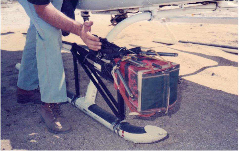
FIGURE 4. —The skid-mounted net gun loaned by Mel Cain to Don Landells and used to capture bighorn sheep. It was a hand-held model, but Don Landells constructed the external mount to secure it to the right skid of the Jet Ranger helicopter so that the pilot could “aim” the net gun at the target animal and then fire it. Note the recoil-absorbing spring located immediately behind the canister and below the Enfield receiver (photo by Charlie Jenner).
