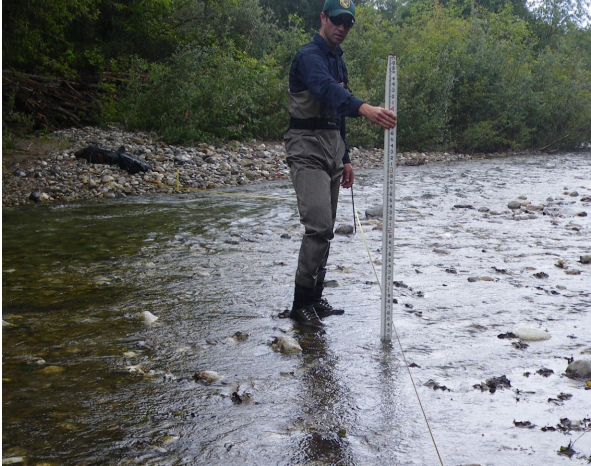
Figure 2. Example using stadia rod to measure depth along a critical riffle transect
