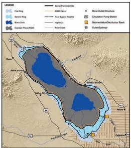
desert pupfish. The inner ring, or second ring, would be a marine waterbody with a maximum depth of 10 feet that would provide additional shoreline habitat. Both rings would be created by constructing rockfilled dikes or levees (Perimeter Dikes).
