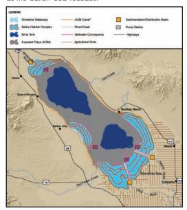
**Alternative 3, Concentric Rings:** The Concentric Rings Alternative would preserve the Salton Sea's existing shoreline habitat by constructing two concentric water bodies. The outer waterbody, or first ring, would be a brackish waterbody ranging from 0 to 10 feet deep that would preserve the existing shoreline habitat and provide connectivity for the
