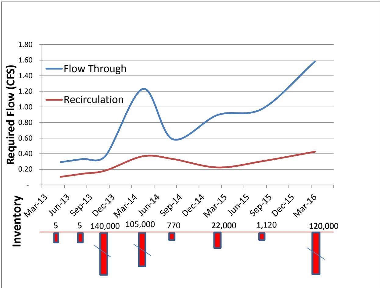
Figure 1. Flow requirements at the Interim Facility for flow-through versus recirculated water.
