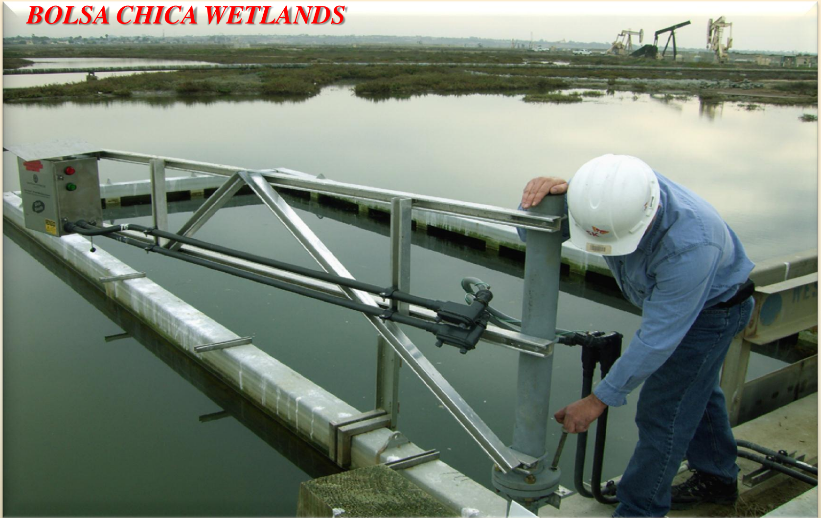
Example of Mounting Sensor on Swinging Adjustable Deployment Arm
