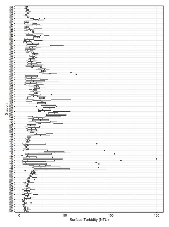
Figure 5. Distribution of monthly surface turbidity (NTU) recorded during the 2021 FMWT season. Boxplots show the median as a vertical line, 1st and 3rd quartile by a box, range by a horizontal line, and outliers by points.
