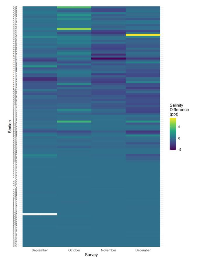
Figure 13. Heatmap of salinity (ppt) differences between surface and bottom water recorded during the 2021 FMWT season. White values indicate missing data. Negative (blue to purple) values are higher salinity on the bottom compared to the surface. Positive (green to yellow) values indicate higher salinity at the surface.
