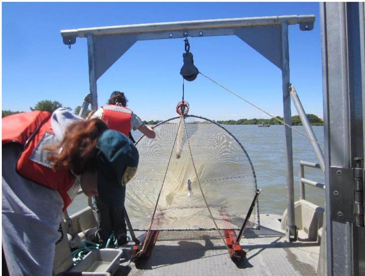
*Figure 2. The Summer Towner sled ready to be deployed. Note the meso-zooplankton (Clark-Bumpus) net mounted at the top of the D-ring and the flowmeter mounted in the center of the main fish net.*
