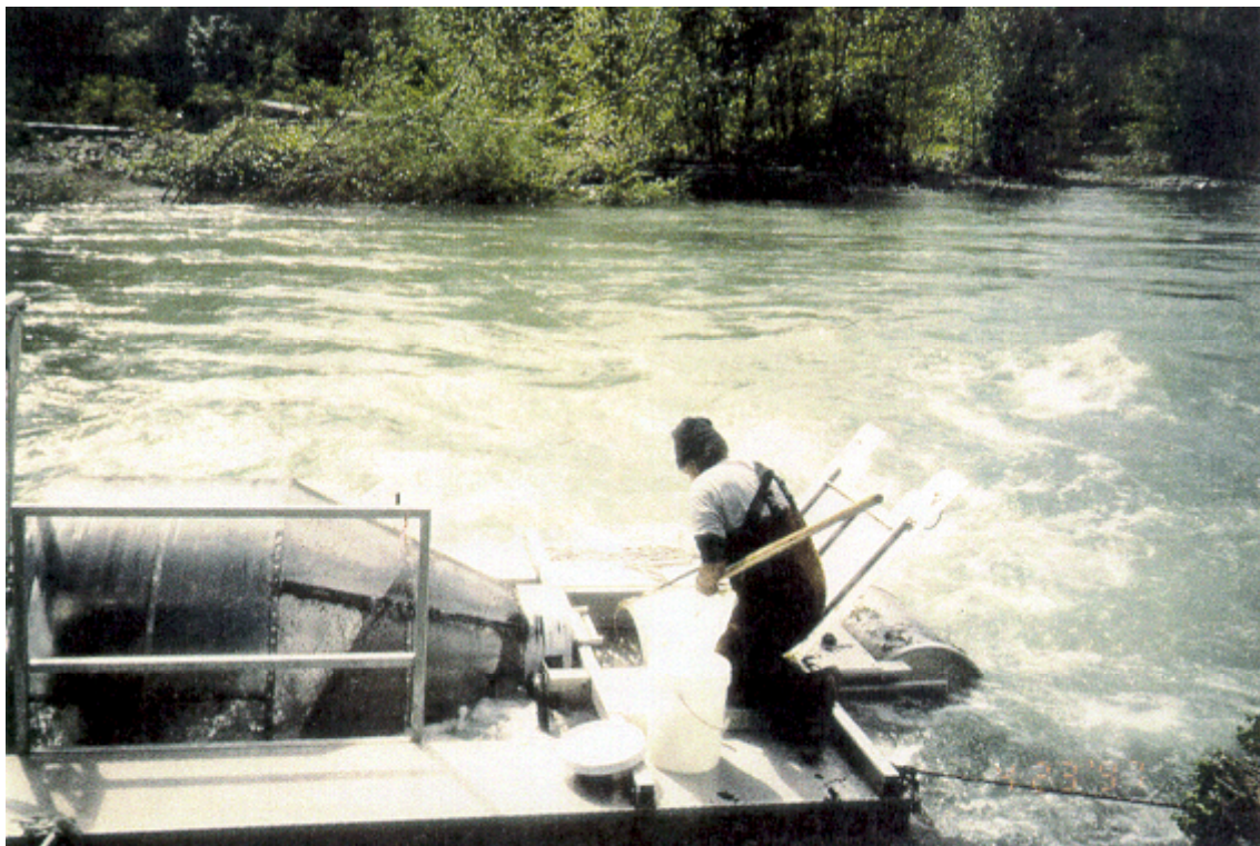
Plate 5. YTFP staff retrieving fish captured in the rotary screw trap, Blue Creek, lower Klamath River, California, 1997.
