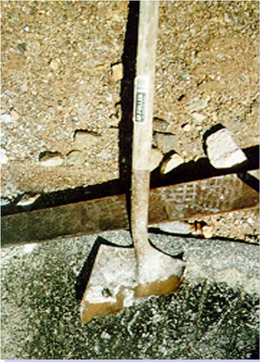
Photo 5: According to EPA documents, workers once inadvertently left a shovel standing in the green liquid flowing from one of the mine portals. The next day half of the shovel had been eaten away.
