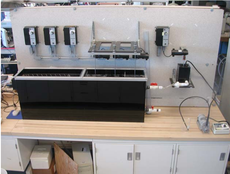
Photo 1. The coagulation, flocculation, sedimentation (CFS) unit.
