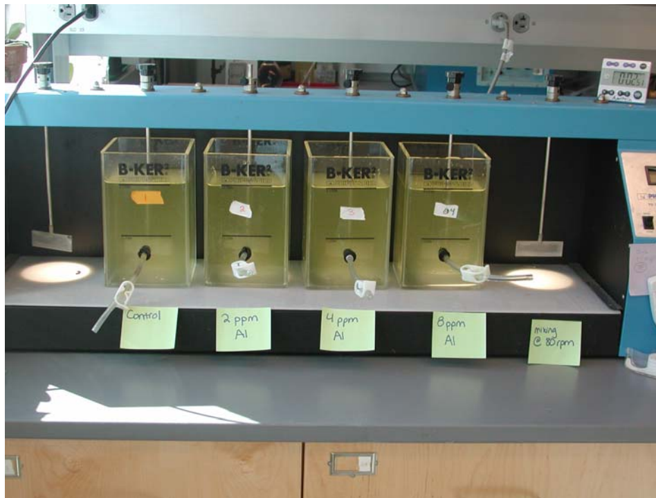
Photo 5. Phipps & Bird 2L jar tester apparatus with CEP water during initial mixing stage.
